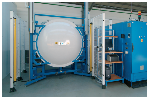
SF 6 filling and sealing station
