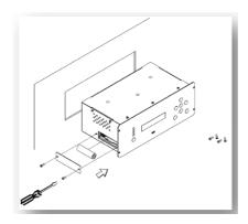
7. Put the relay into the RMU switchgear and tighten the 4 screws on the front to fix the relay.
