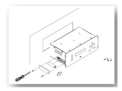
5. Remove the battery and replace it respecting polarity (+ facing up):
