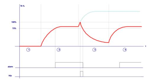
Supposing that thermal image protection has an adjusted tap of 1,1 times the nominal current and an alarm level of 75%:
