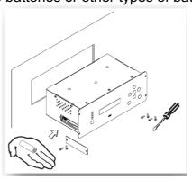
6. Put on the battery cover and tighten the 2 screws.
