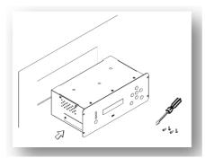
4. Unscrew the 2 screws to remove the cover from the battery compartment.
