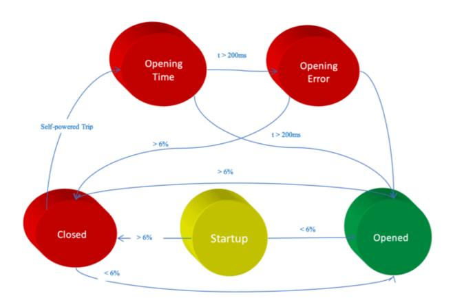
If both of the circuit breaker contacts 52a and 52b are available, they should be wired to the two physical inputs. These physical inputs are then assigned to the corresponding logic signals: the circuit breaker 52a contact to the "52a" logic signal, and the circuit breaker 52b contact to the "52b" logic signal. The circuit breakers automaton is considered as having eight statuses: Start, open, closed, error, opening time, opening error, closing time and closing error.
