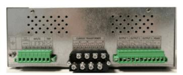
The other terminals (inputs, outputs, communication and auxiliary power supply) are designed for 24 AWG - 12 AWG cable: 0.25 - 2.5 mm2 with a tightening torque of 0.5 Nm-0.6 Nm.
