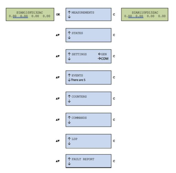
Press the "OK" key to access the second level from the main screen. Use the ▲ and ▼ keys to move from one menu section to another in the second level. Use the "C" key to return to a higher level.
