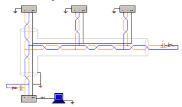
Minimum required current to achieve remote communication: 360 mA (single phase), 180 mA (2-phase) and 120 mA (3-phase).
