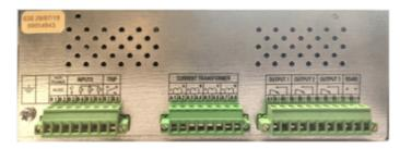
Option 2: Rear power supply terminals with ring clamps (12 AWG - 22 AWG: 4 - 0.3 mm2 cable with torque of 0.79 Nm - Model SIABxxxxx7xx):
